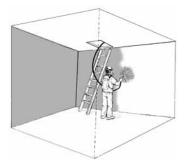
This water cistern is a confined space with limited access and ventilation. While a waterproof coating was being applied, flammable vapours were generated. The vapours ignited, and an explosion occurred. One worker died, and another was severely injured.
