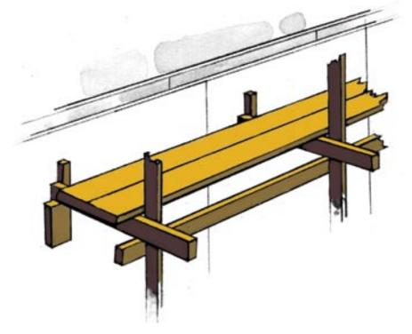
Single-pole wooden scaffolding for pouring or pumping concrete. Note: Guardrails may not be required if scaffolding is less than 3 m (10 ft.) above grade.
