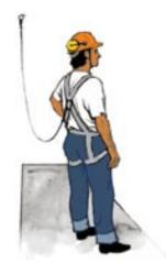
This is an example of a fall arrest system. Fall arrest systems protect workers after they fall by stopping the fall before they hit the surface below.
