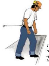
This is an example of a fall restraint system. Fall restraint systems prevent workers from falling.
