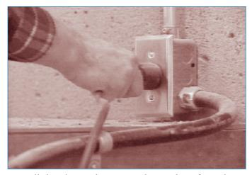
Pull the plug to disconnect the machine from the electric power supply.
