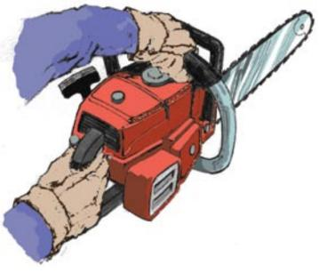
Diagram showing proper grip of a chainsaw
