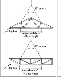
Trusses up to 9 m (30 ft.) in length should be lifted using two pickup points so that the distance between them is approximately one-half the length of the truss.
