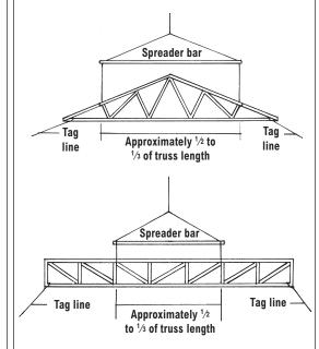
A spreader bar and short wire rope slings should be used to lift trusses 9–18 m (30–60 ft.) long. The slings may be vertical or may toe-in. Two tag lines should be used to control the raising of trusses of this size.
