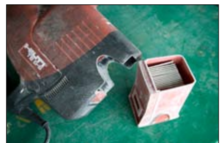
Drill with dust removal system
