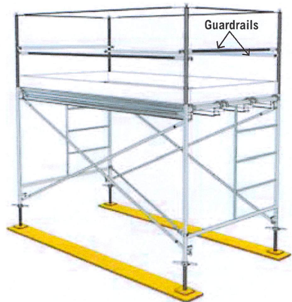
This is an example of a metal guardrail system.
